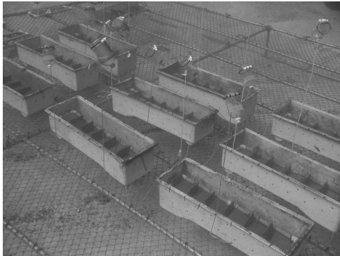
Figure 2: Coral recruitment platform constructed on a sand patch on the East Flower Garden Banks at 24m depth.
